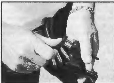
With the muzzle down, rounds are fed into the chambers two at a time from the Speed Strip. The cylinder latch is opened, and the now-loaded cylinder is closed.
